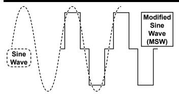
This Inverter's output is a Modified Sine Wave.
