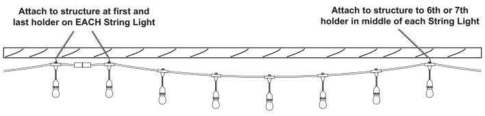
2. If attaching to guide wire, attach the ring at the back of **every bulb holder** to the guide wire using a S-hook or cable tie (sold separately).
