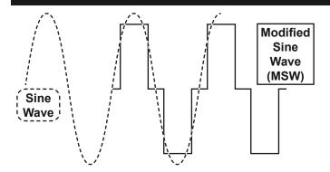
1. This Inverter's output is a Modified Sine Wave. Power from most electric utilities is a Sine Wave.
