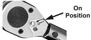
**Note:** Thread fastener with another tool until it is just snug, then finish the operation with the Torque Wrench.
