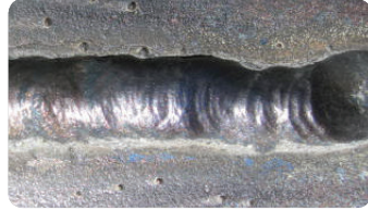
Weld Speed Too Slow
