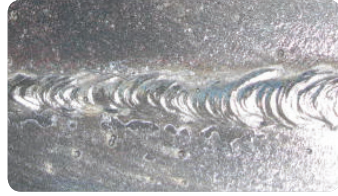
Current Too High or Wire Feed Too Fast
