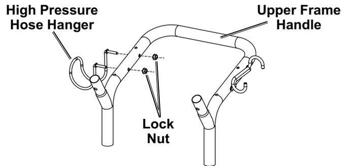
2. Slide the Upper Frame Handle (14) over the two upright tubes on the Frame (2) and press down until Handle is seated and two Detent Pins snap into place.
