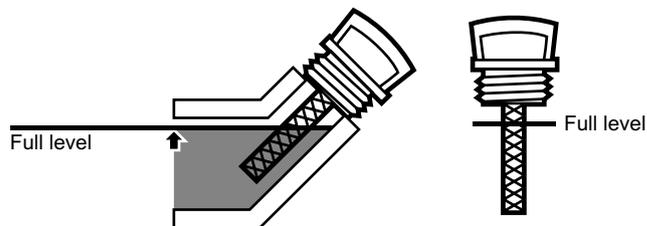
4. Reinsert the Dipstick without threading it in and remove it to check the oil level. The oil level should be up to the full level as shown above.
