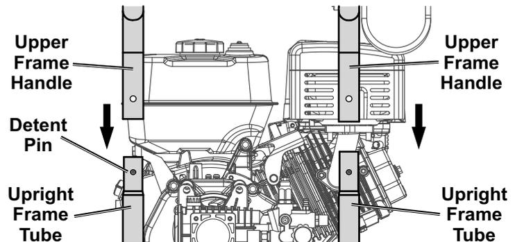
3. Slide the Front Frame Handle (20) over the two angled tubes on the Upper Frame Handle and press down until Handle is seated and two Detent Pins snap into place.
