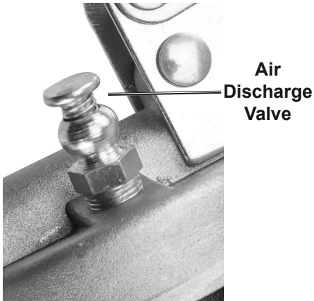
Figure A: Air Discharge Valve location
