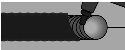
PARTIALLY CHIPPED AWAY TO SHOW WELD
