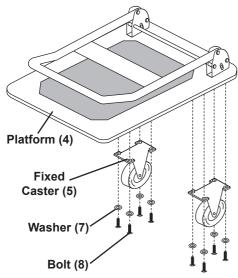
Attach the Fixed Casters (5) to the Platform (4) near the Handle Bracket (3) using Washers (7) and Bolts (8).
