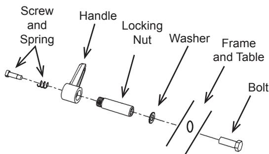
Figure F: Installing Handle
