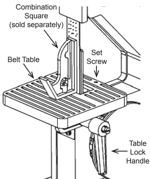
Figure G: Adjusting the Belt Table
