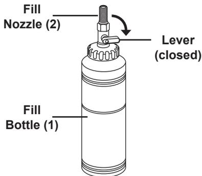
**Figure A: Fill Bottle and Fill Nozzle**
