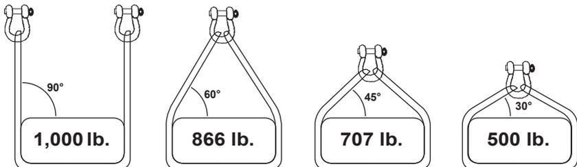
A sling capable of lifting 1,000 lb. In a 90° vertical basket hitch can only lift 866 lb. at a 60° angle, 707 lb. at a 45° angle, and 500 lb. at a 30° angle.
