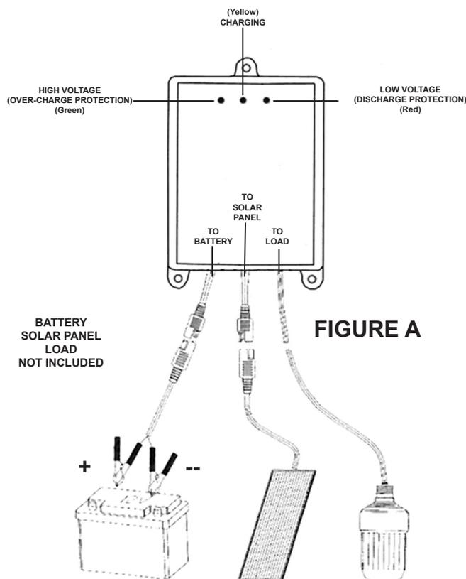
2. When a solar panel is connected to the Charge Regulator, the **YELLOW** (charging) LED light will illuminate to show that the 12 volt DC battery is receiving charge from the solar panel. **(See Figure A.)**
