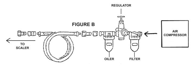
3. Connect a compressed air supply hose (not included) to the previously installed Quick Connector. Then turn on the air compressor, and set its regulator to 90 PSI. Do not exceed 90 PSI. (See Figure C.)
